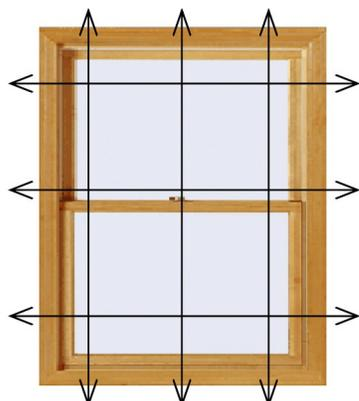
Step 1. Measure the width of the area you wish to cover. Measure in 3 places across the top, center and bottom of the window. Record the largest of the 3 measurements. We recommend adding overlap to reduce light leakage around the See *Recommended Overlap*. This is your ordering width.
