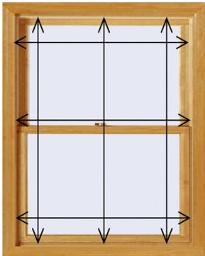
Step 1. Measure the width of the opening at the top, middle, and bottom of window. Record the narrowest of the 3 measurements. This is your ordering width. The factory will make the necessary deductions to ensure a proper fit. **DO NOT TAKE A DEDUCTION.**
